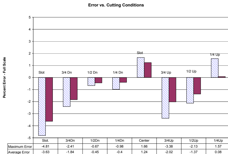
Figure 7 Shows the Maximum and average full scale percent error for eight different cutting conditions. The errors are maximum and average for four different feedrates for each of the eight cutting conditions using the average value of ten samples per condition.
